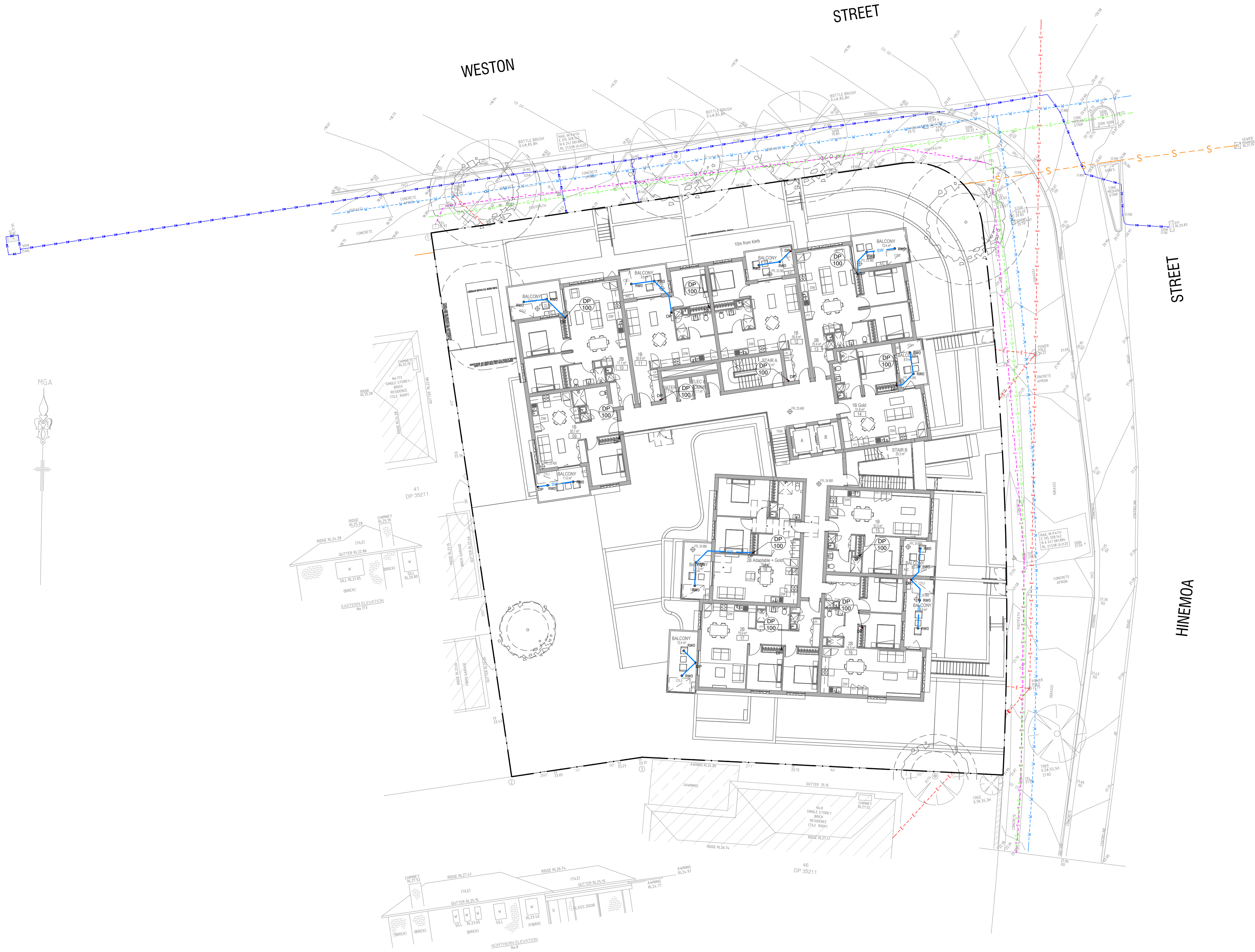
FIRST FLOOR STORMWATER DRAINAGE PLAN
